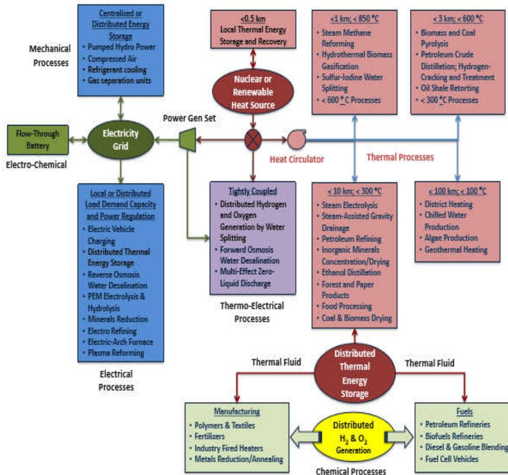
Figure 8. Summary of potential N-R HES applications indicating energy conversion varieties possible and their appurtenant processes. Developed by: Idaho National Laboratory (US DOE, 2015)
