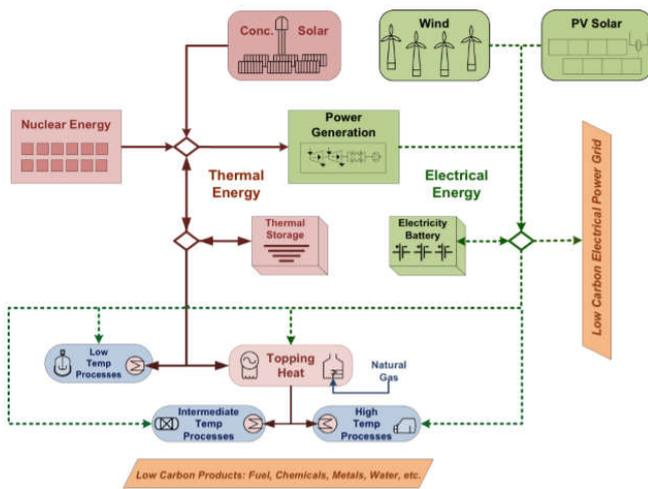
**Figure 5. General architecture for a tightly coupled nuclear renewable hybrid energy system, developed by Idaho National Laboratory (US DOE, 2015)**
