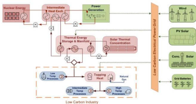
**Figure 6. General architecture for a thermally coupled nuclear renewable hybrid energy system, developed by: Idaho National Laboratory (US DOE, 2015)**
