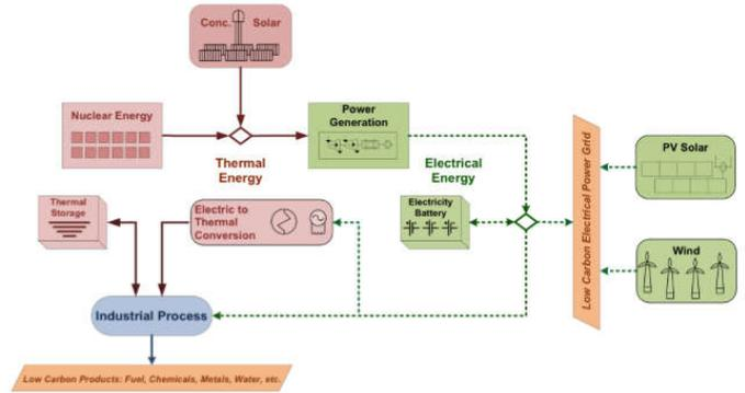
**Figure 7. General architecture for a loosely coupled (electricity only) nuclear renewable hybrid energy system, developed by: Idaho National Laboratory (US DOE, 2015)**
